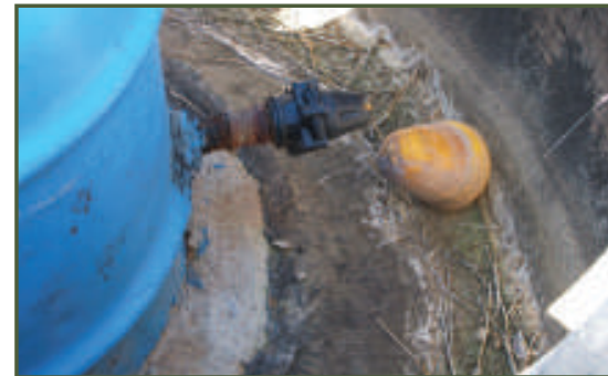
Waterline empties into the trough with a quick coupler and float.
